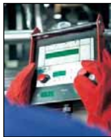
3. Just the word 'remote control' says it all. Each parameter can be operated and controlled in a distance of up to 25 metres from the power source.
