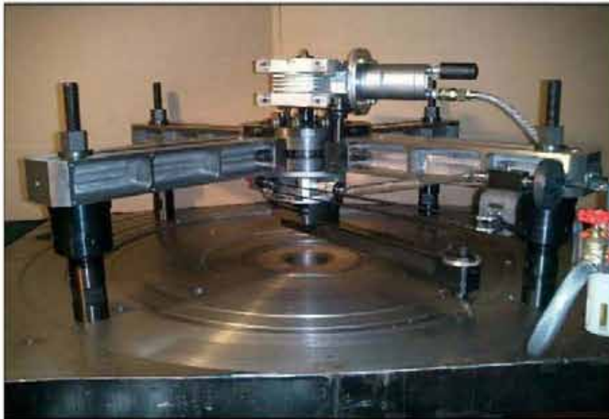
SERCO XP 1200 / XP 1800 / XP 2000 / XP 2200 PORTABLE EXTRA FLAT FLANGE FACING MACHINE
